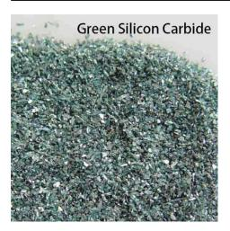
**Green Silicon Carbide** is produced from quartz sand and petroleum coke in a high-temperature electric furnace. It features **purity above 99.5%**, high hardness, and excellent chemical stability.
