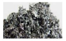
Zirconia Alumina is a synthetic high-hardness abrasive known for excellent hydrophilicity and electrostatic properties, widely used in grinding, polishing, and sandblasting.
